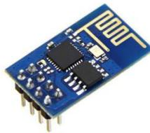
Figure 2: WIFI MODULE-ESP 8266
