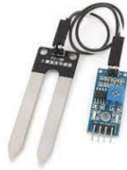
Figure.4: SOIL MOISTURE SENSOR-FC28
